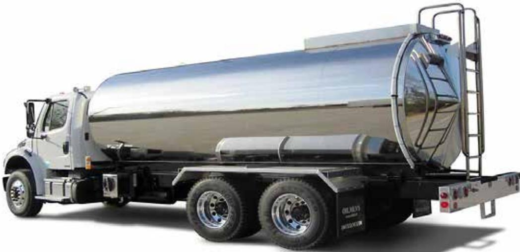
Bulk raw milk transport tankers should be appropriately designed, constructed and insulated. The raw milk contact surfaces should be made of stainless steel. It should be cleaned and sanitized before use. Other requirements include:
