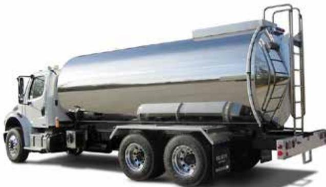
**Bulk raw milk transport tankers should be appropriately designed, constructed and insulated. The raw milk contact surfaces should be made of stainless steel. It should be cleaned and sanitized before use. Other requirements include:**
