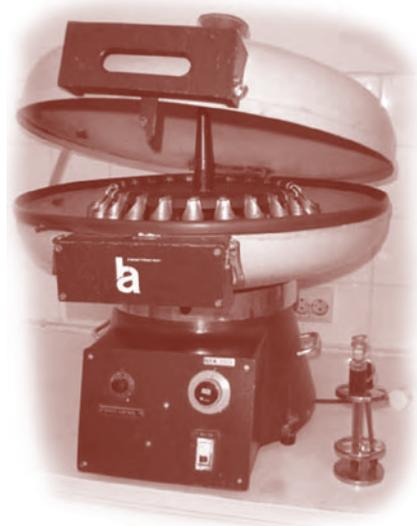
Apparatus for carrying out Gerber butterfat test
